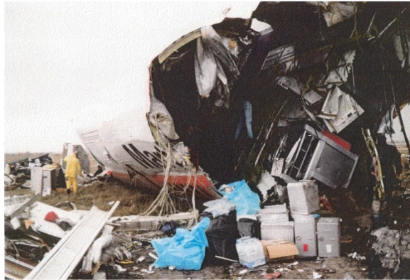
View of the rolled over and broken off front part of the crashed Anthony Ruys
